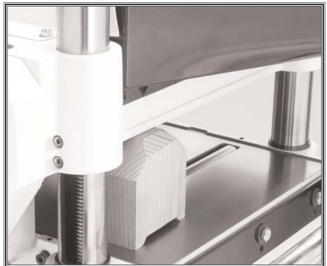
Figure 14. Checking cutterhead alignment.
